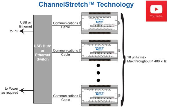
\*DATAQ Instruments 7-port USB hub (part number 2000310). Cascade for a higher port count.
