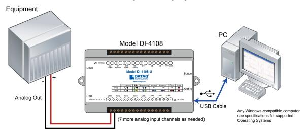
Examples of "Equipment" above include gas chromatographs, liquid chromatographs, spectrometers, bio-amplifiers\*, etc.
